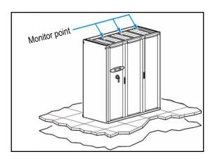
Figure 3 – Cooling system return air humidity monitoring
