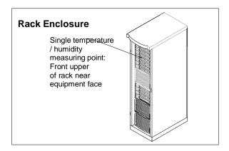
Use a temperature-humidity probe that interfaces with currently used operating and control systems to monitor and provide proactive warning of out-of-range humidity conditions (**Figure 2**). Many hand-held monitoring devices available that allow for spot-checking of temperature and relative humidity anywhere in the room.
